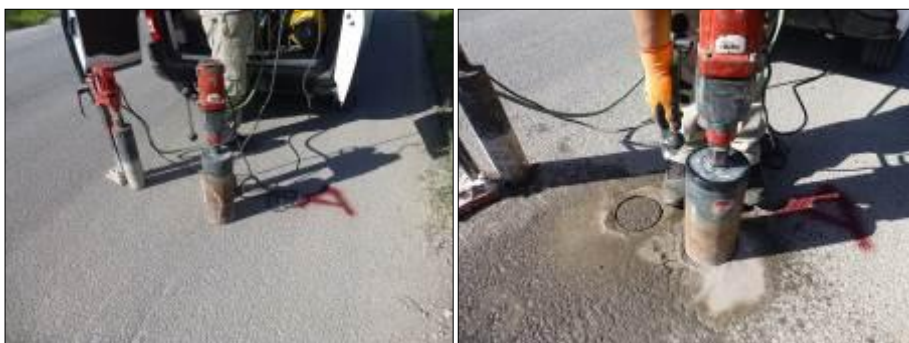
Figure 7. Field core drillers of 100 and 150 mm diameter and drilling two 150 mm core pair at location A
