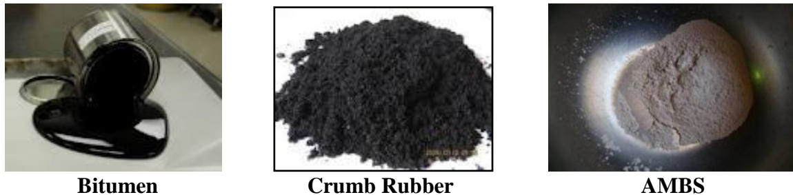
Figure 1: RAR ingredients: Asphalt Cement (Bitumen), Crumb Tire Rubber and AMBS
